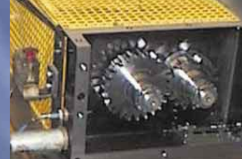
FZG Gear test rig to test the load carrying capacity of EP/AW gear oils and lubricating oils
