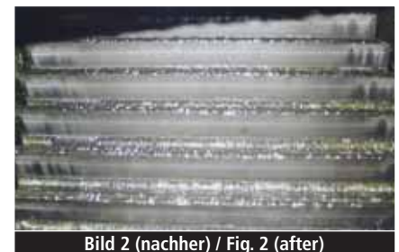
Gutes Breitentragen. Good contact pattern over the whole tooth flank.
